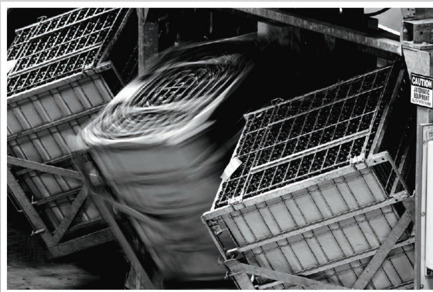
Robotic gyro-palletes are the industry standard for riddling sparkling wines, but researchers are working on an alternative method. Photo: J Vineyards & Winery
